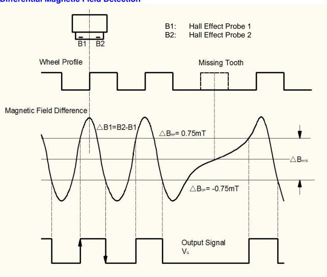
Operating point: B2-B1 <  $\Delta B_{OP}$  switches the output ON (V<sub>Q</sub> = LOW) Release point: B2-B1 >  $\Delta B_{RP}$  switches the output OFF (V<sub>Q</sub> = HIGH)
