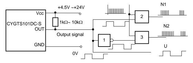
The target wheel rotates in the counter-clockwise direction if N1 < N2. Otherwise the target wheel rotates in the clockwise direction (N1>N2). The rotational speed can be determined by (4) under using the pulse signal U. In order to guarantee the detection of the rotational direction, the condition Q>2P should be fulfilled.
