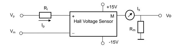
A magnetic field is generated by current  $I_p$  when a voltage  $(V_p-V_m)$  is applied to the input terminals of the sensor through the primary resistor  $R_i$ . This magnetic field is compensated with the reverse magnetic field caused by the current  $I_s$  in the secondary coil. The rest magnetic field after compensation effect can be detected with a Hall Effect element. One obtains the following equation when the magnetic flux is zero:
