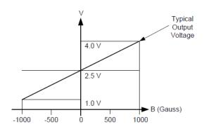
a slight loss of output symmetry. So, it is not recommended to work in such condition unless the output voltage magnitude is a main issue. The output signal can be capacitively coupled to an amplifier for boosting further if the changing frequency of the magnetic field is high.
