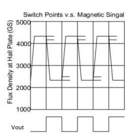
In the case of Ferromagnetic toothed wheel application the IC has to be biased by the south pole of a permanent magnet (Maximum 4000Gs). When assembling the sensor system, suggest to choose a magnet as back bias flux from 1000Gs to 4000Gs. Normally the South pole of magnet faces the unbranded side of the IC. The magnet should be glued to the back surface (non-branded side) of the IC using an adhesive or suitable epoxy. The sensor CYGTS9801 is "self-adjusting"
