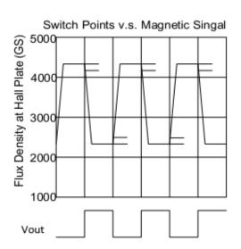
In the case of Ferromagnetic toothed wheel application, the IC has to be biased by the south pole of a permanent magnet (Maximum 4000Gs). When assembling the sensor system, suggest using a magnet as back bias flux from 1000Gs to 4000Gs. Normally the South pole of magnet faces the unbranded side of the IC. The magnet should be glued to the back surface (non-branded side) of
