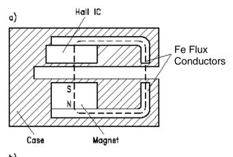
a) Magnetic flux through the Hall-effect switch with no vane in the gap
