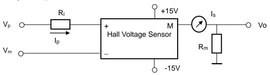
A magnetic field is generated by current  $I_p$  when a voltage  $(V_p\text{-}V_m)$  is applied on the input terminals of the sensor through the primary resistor  $R_i$ . This magnetic field is compensated with the reverse magnetic field caused by the current  $I_s$  in the secondary coil. The field compensation effect can be detected with a Hall Effect element. One obtains the following equation when the magnetic flux is zero:
