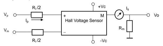
Polarity: output current I<sub>s</sub> is positive when input current I<sub>p</sub> is applied on the "+" terminal
